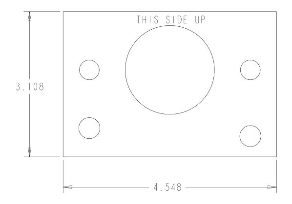
INSTRUCTIONS: CUT OUT TEMPLATE INCLUDING ALL 5 HOLES. THIS TEMPLATE SHOULD LAY FLAT ON FIREWALL AND ALL HOLES SHOULD LINE UP. IF SO, HYDROBOOST BRACKET WILL WORK.VERIFY BOTH DIMENSIONS ARE ACCURATE AFTER YOU PRINT TEMPLATE.
